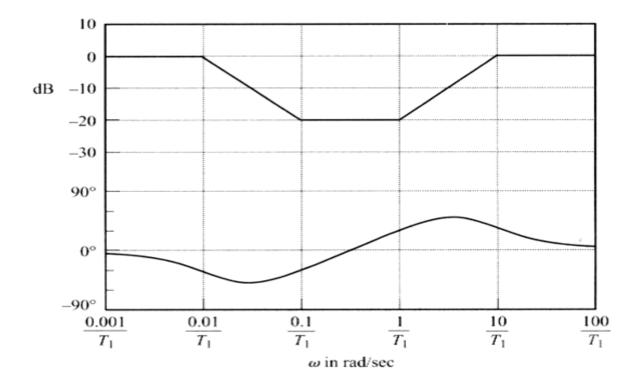
Example Lag-Lead design; Desired system is K<sub>v</sub> of 10 sec<sup>-1</sup>, PM is at least 50° and GM is at least 10 dB
